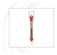
A spring scale or spring balance is a type of weighing scale. It consists of spring fixed at one end with a hook to attach an object at the other.
